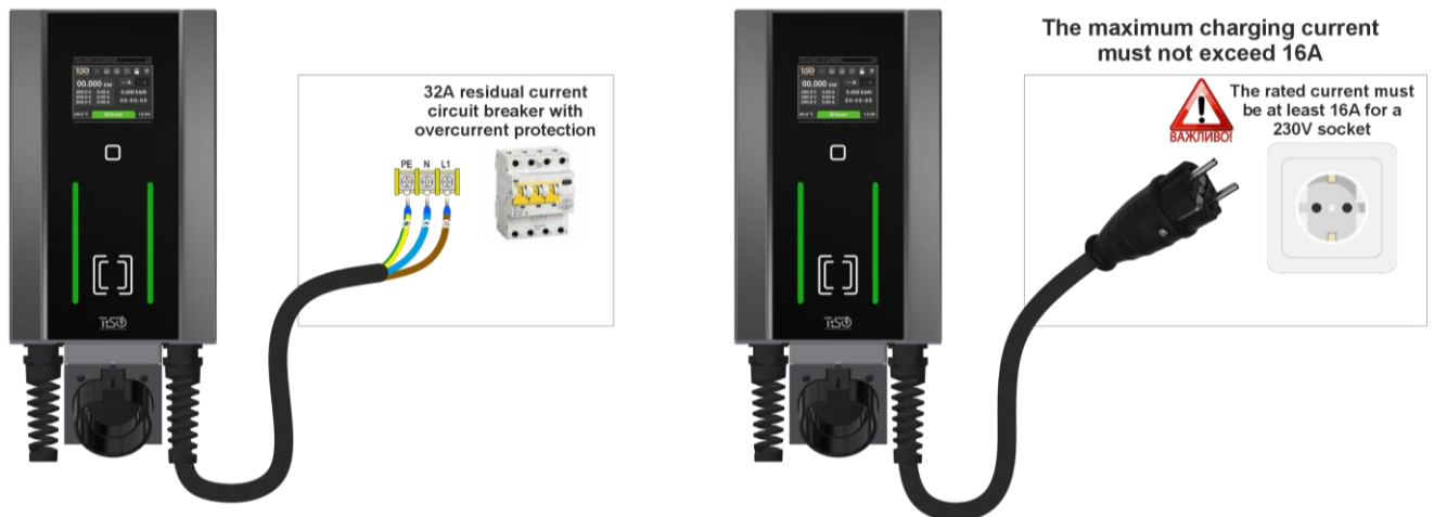
Fig. 8 - Single-phase charging station connection options
